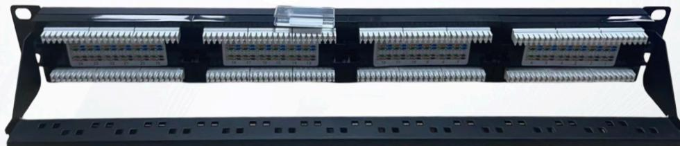
1U 19" 24 Port CAT6 Patch Panel is designed for high-performance and organized network infrastructure in data centers and enterprise environments. Featuring 50µm gold-plated contacts, it ensures superior conductivity and durability. The built-in cable management bar provides a clean and secure way to manage cables
