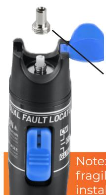
Rotate counterclockwise to remove the visual fault locator Front end metal head The ceramic core can be replaced. Replacing the metal head Tighten with proper force
